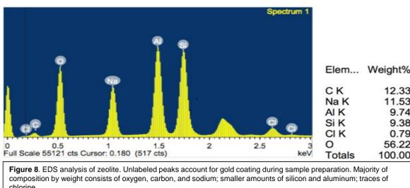
Figure 8. EDS analysis of zeolite. Unlabeled peaks account for gold coating during sample preparation. Majority of composition by weight consists of oxygen, carbon, and sodium; smaller amounts of silicon and aluminum, traces of chlorine.
