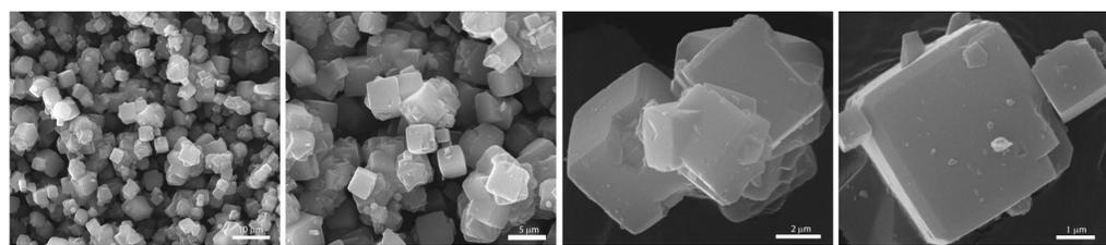
Figure 7. Scanning electron microscopy imaging of Zeolite at increasing magnification. Note cube-like structure and particle size of approximately 1-3 microns.
